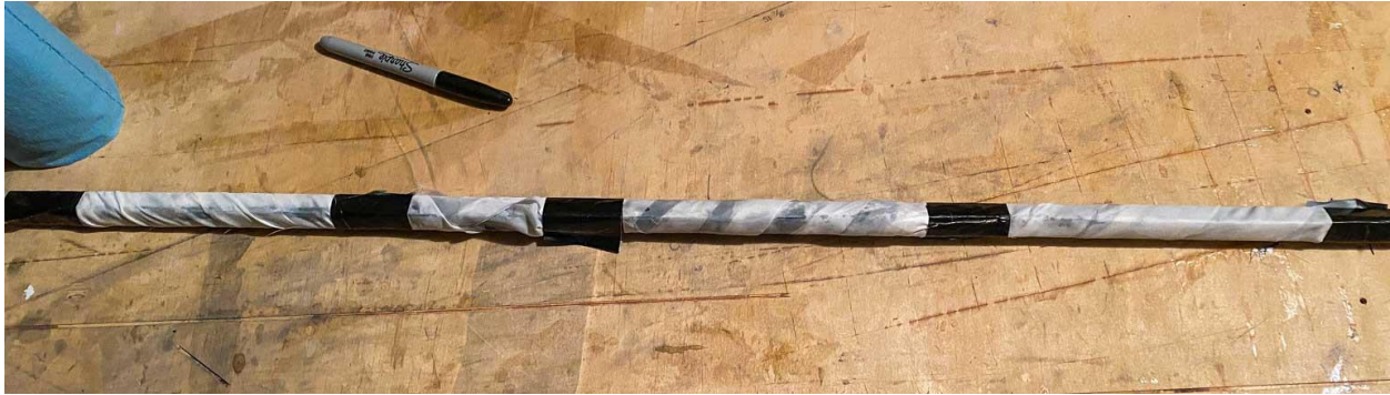
Above: "Glued" carbon fiber pieces held together with peel-ply & duct tape
