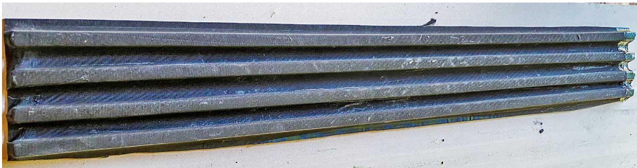
Above: After vacuum bagging using wood 36" mold pieces
