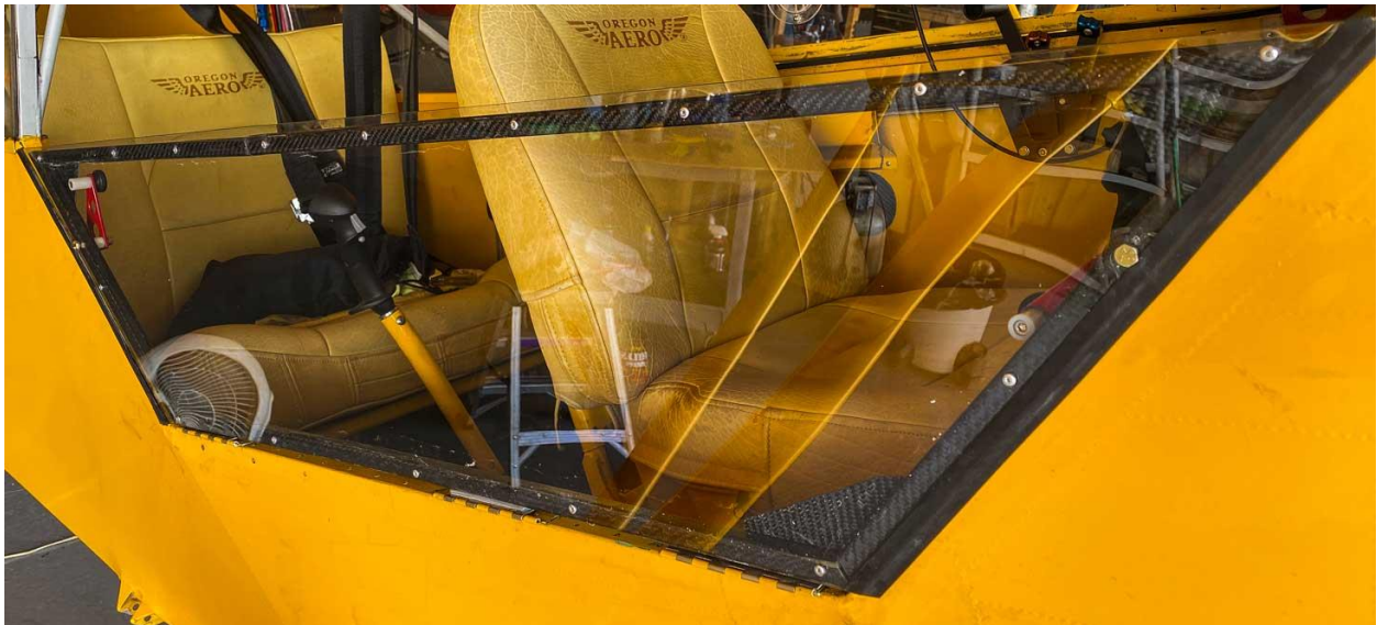
Above: First door/window in place (lots of reflections from new Lexan)
