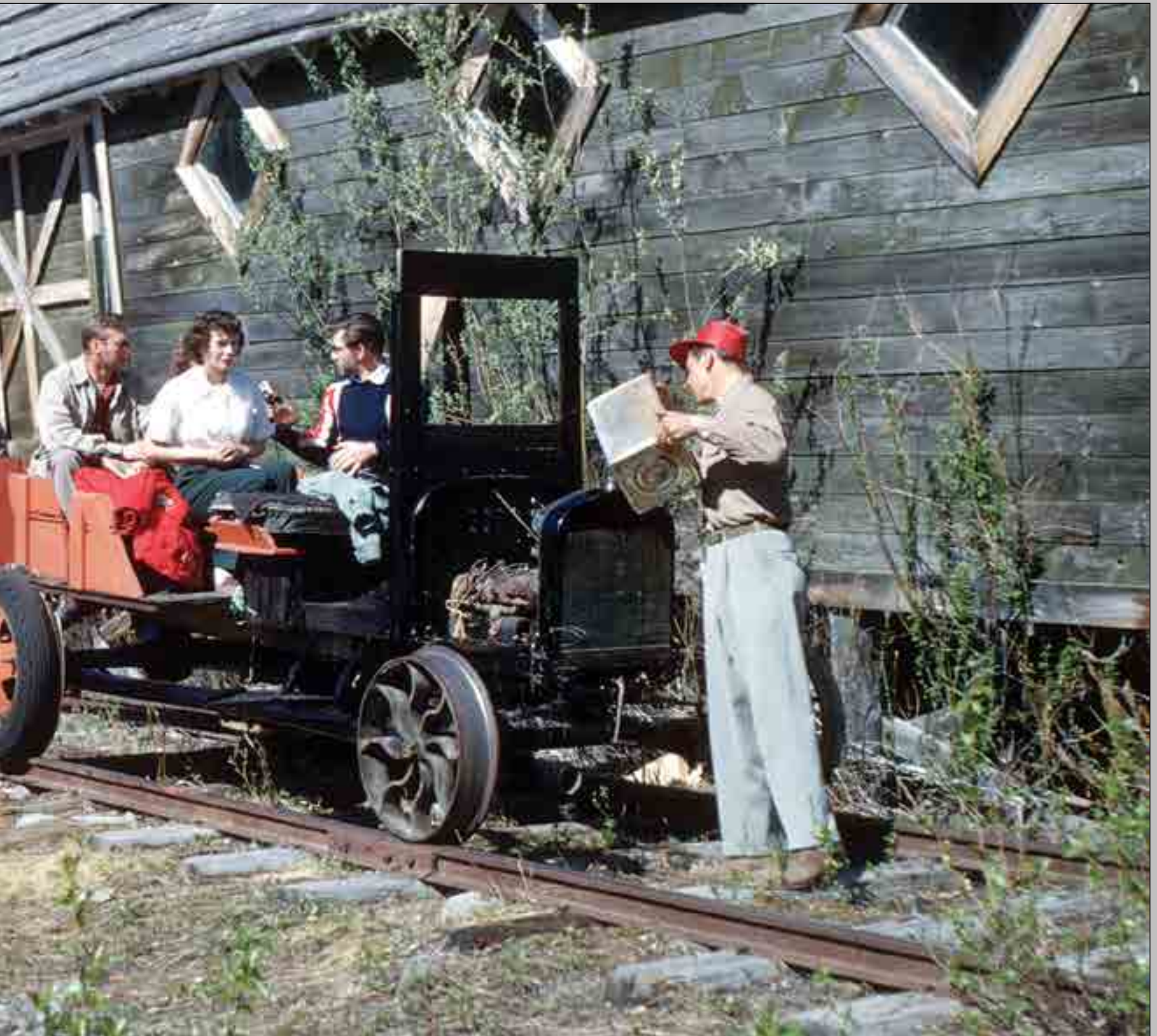
On the second day of the Sourdough Tour, visitors made the six mile trip to Kennecott for a picnic and to hike around. Travel between McCarthy and Kennecott took place on The “Kennecott Express,” a Model T automobile mounted on railroad wheels that pulled tourists riding in wooden rail carts around the deserted structures. Cordova Airlines pilot Howard Knutson preparing tourists for the featured ride on the “Kennecott Express.” Courtesy of Charles “Bob” Leitzell.
